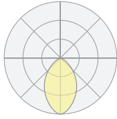
Lambertian 0.375" Frosted Regressed Lens
